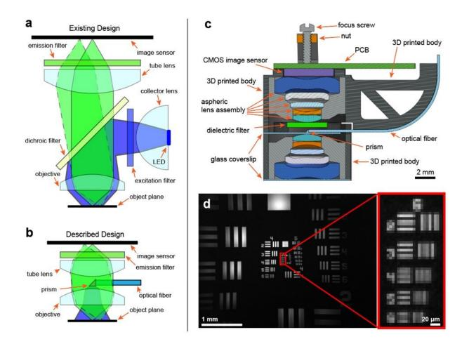
A schematic of the components of standard head-mounted microscopes (a) and the new design (b-c), which eliminates the standard illumination optics resulting in a device that is significantly more compact and lightweight. Panel (d) shows that the microscope retains high resolution, with the ability to distinguish lines
