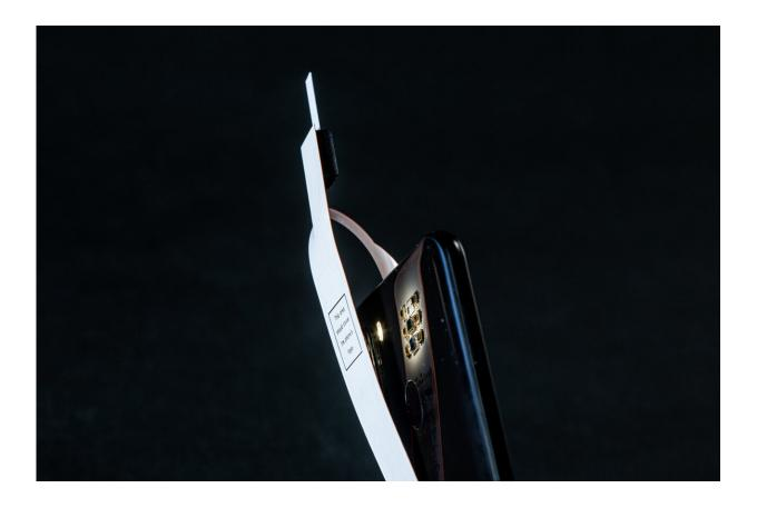
Researchers at the University of Washington have developed GlucoScreen, a system that could enable people to self-screen for prediabetes. It uses a modified version of a commercially available test strip (white rectangle) with any smartphone—no separate glucometer required. Tiny photodiodes on the GlucoScreen test strip enable it to draw the power it needs to function entirely from the phone's flash—no batteries or USB connection required. Credit: Raymond C. Smith/University of Washington
