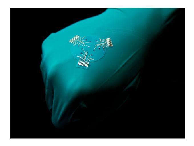
A larger version of the smart bandage rests on the back of a gloved hand. Credit: Caltech
