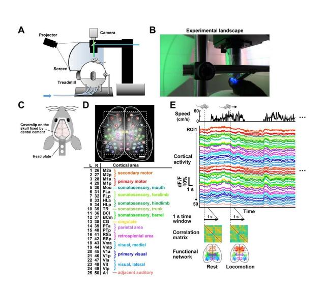
Figure 1. A, The imaging and virtual reality (VR) system. B, Photograph of the experiment C, A schematic of the transcranial imaging window affixed to the mouse skull. D, Fifty cortical ROIs are overlaid onto a grayscale image of the dorsal cortex with a cortical parcellation map (top, dashed lines indicate the field
