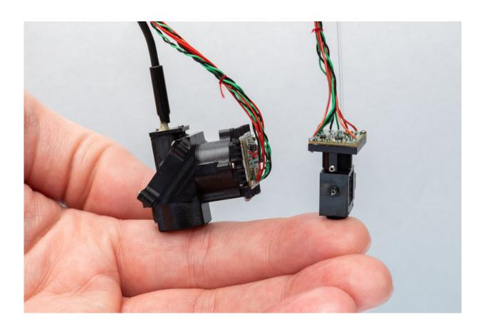
Salk researchers developed two wearable microscopes to image cellular activity in previously inaccessible regions of the spinal cord of moving mice in real-time. Credit: Salk Institute
