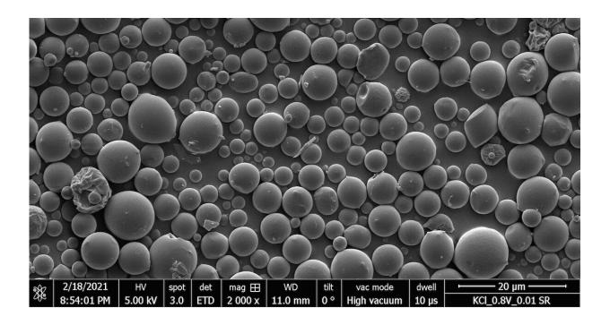
Scanning electron micrograph of biodegradable microparticles that reprogram immune cells to protect joints against inflammatory arthritis. Imaged at UC San Diego's Nano3 facility, Jacobs School of Engineering. Credit: David McBride, UC San Diego
