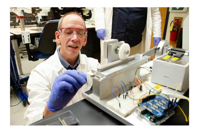
WVU researcher Loren Rieth demonstrates the electromechanical tester that can be used to characterize the lifetime of electrical leads connecting neural electrodes to stimulators. Credit: WVU Photo/Paige Nesbit
