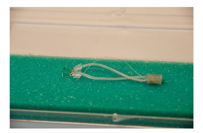
The chronically implantable MouseFlex, developed at West Virginia University, device features specialized leads and connector systems. Credit: WVU Photo/Paige Nesbit
