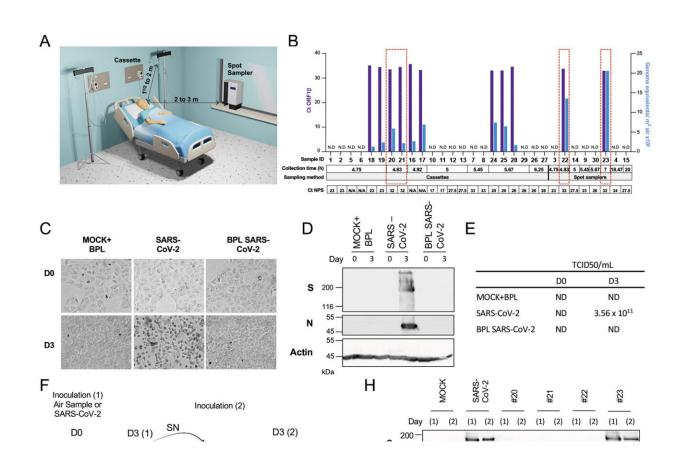
A) Hospital room of patient with COVID-19 layout depicting the position of the sampling devices and the distance to the head of the patient. SKC 37mm closed-face cassettes allow efficient cut off for sampling aerosol and not droplets. They were used pointing downward to prevent accidental contamination by droplets. The Series 110A Liquid Spot Sampler Spot Sampler collects small-size aerosols of 5nm to 10 $\mu$ m. B) Quantification of SARS-CoV-2 ORF1 $\beta$  RNA by RT-qPCR
