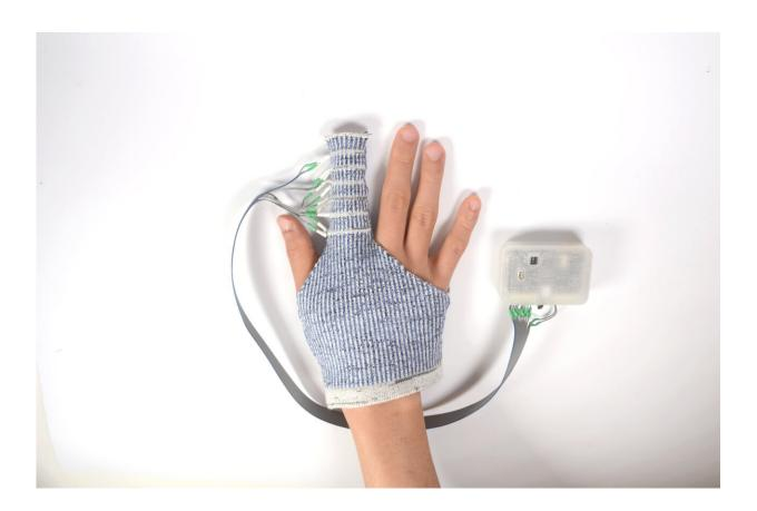
KnitDema consists of machine-knitted semi-glove and hardware to compress edematous hands sequentially. The device covers the index finger and uses embedded shape memory alloy (SMA) bands to mobilize edema fluid from the fingertip to the base. Credit: Hybrid Body Lab
