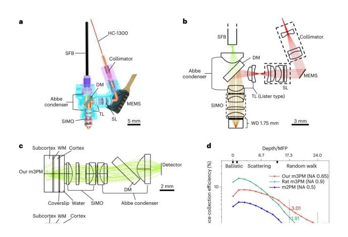
Optical configuration of the miniature headpiece maximizing scattered fluorescence collection. Credit: *Nature Methods* (2023). DOI: 10.1038/s41592-023-01777-3
