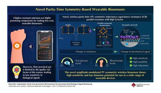
Researchers have developed a novel, wireless, PT-symmetric wearable resonator that can detect tear glucose and blood lactate levels in the micromolar range. The resonator is composed of an inductance–capacitance–resistance (LCR) reader and an LCR sensor with an enzyme-based chemiresistor. The setup has a high quality (Q) factor, making it highly sensitive. Credit: Professor Takeo Miyake from Waseda University
