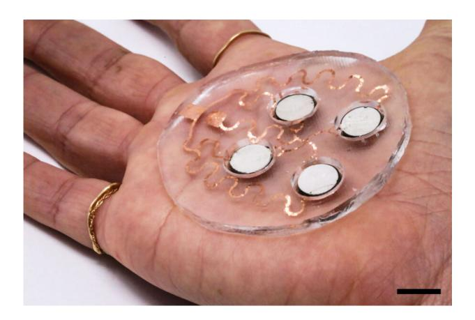
MIT researchers have developed a wearable patch that applies painless ultrasonic waves to the skin, creating tiny channels that drugs can pass through. Credit: Chia-Chen Yu et al
