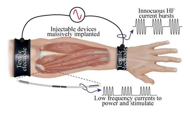
Working principle of the intelligent wireless network of sensors and actuators consisting of injected electrodes and external textile electrodes and controllers. Credit: Equinor, Open Data License
