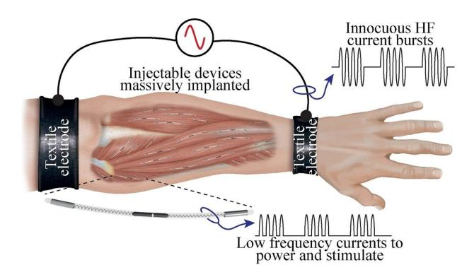
Working principle of the intelligent wireless network of sensors and actuators consisting of injected electrodes and external textile electrodes and controllers. Credit: Equinor, Open Data License
