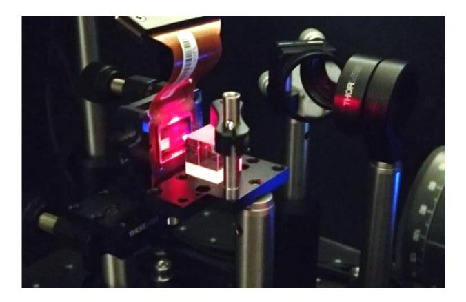
The researchers used a spatial light modulator — shown here being illuminated by the interrogating beam — to reproduce, for the first time, real aberrations produced by different angles of illumination for different myopic eyes. This allowed them to rigorously analyze different types of eyeglass lenses that are used to slow myopia progression. Credit: Augusto Arias-Gallego, ZEISS Vision Science Lab
