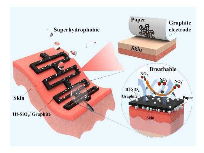
The sensors use a silica hydrophobic coating, which has not been used previously for the pencil-on-paper sensors. These sensors were also designed to be stretchable, making it possible to wear on the skin. Credit: Huanyu "Larry" Cheng
