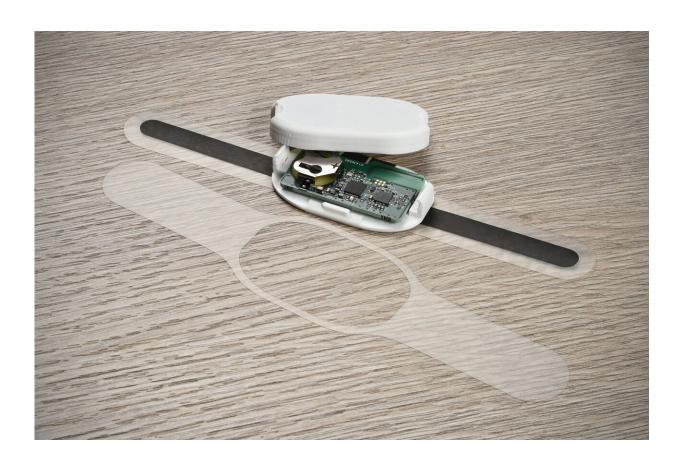
Biodegradable ECG patch in parts. Credit: VTT Technical Research Centre of Finland
