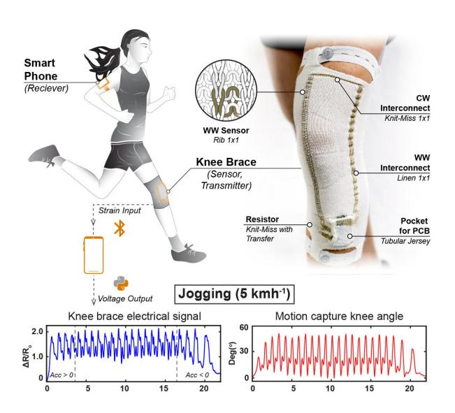
The smart fully knitted knee brace seamlessly integrates multiple flexible electrical components into a stretchable circuit. When worn, the knee brace
