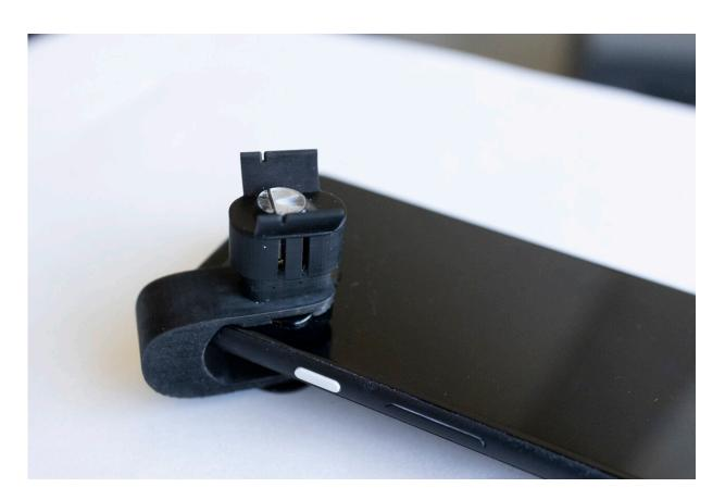
Prototype of the blood pressure monitoring clip. The user presses on the clip and a custom smartphone app guides the user on how hard and long to press during the measurement. Credit: Digital Health Lab / UC San Diego
