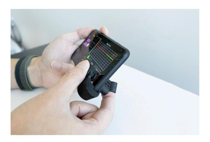
Prototype of the blood pressure monitoring clip. The user presses on the clip and a custom smartphone app guides the user on how hard and long to press during the measurement. Credit: Digital Health Lab / UC San Diego
