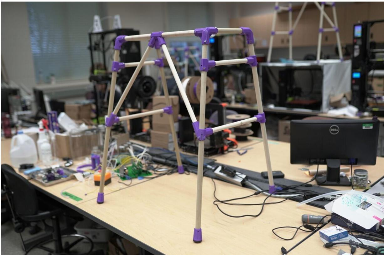
The current walker design should be safely capable of bearing the load of an individual's weight between 78.9 to 93.5 kilograms (approx. 174 to 206 pounds).
