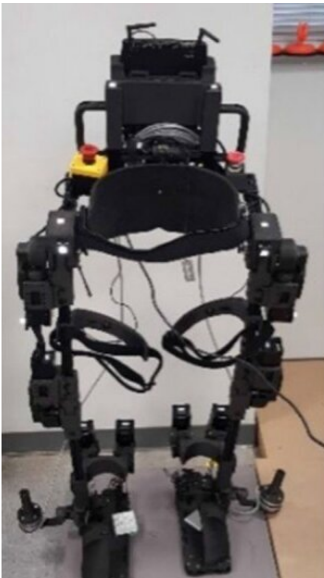
(Left) The developed prototype of the lower extremity robotic exoskeleton (LE-
