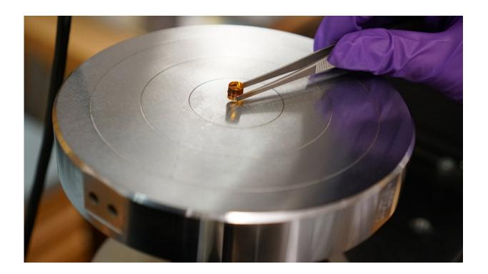
Placing the hydrogel on a compression machine. Credit: Alex Walls
