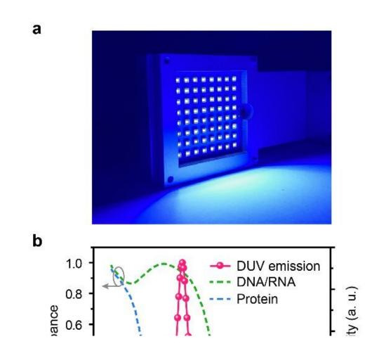
The developed planar light source (a) The DUV solid-state light source comprised of nitride-based LEDs; (b) Electroluminescence spectrum of the fabricated LED chip. The green and blue dotted lines were the standard absorption spectra of DNA/RNA and proteins extracted from published values,
