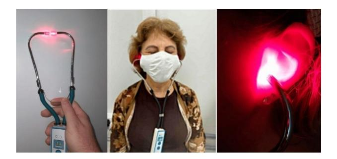
LLLT prototype device applying red laser with a wavelength of 660 nm developed at the Technological Support Laboratory of IFSC-USP for laser auriculotherapy. Credit: *Journal of Personalized Medicine* (2023). DOI: 10.3390/jpm13040581
