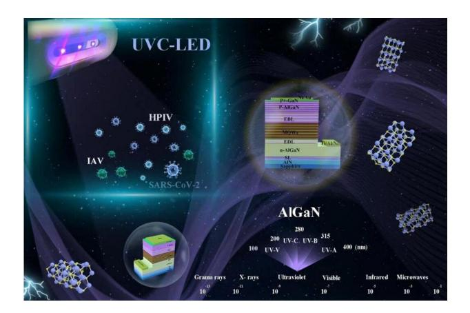
Operating wavelength, typical structure and application in disinfection and sterilization field of AlGaN based DUV LED. Credit: Compuscript Ltd
