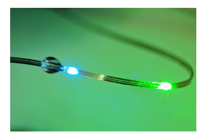
These flexible fibers, which are embedded with sensors and light sources, can be used to manipulate and monitor the connections between the brain and the digestive tract. Credit: MIT
