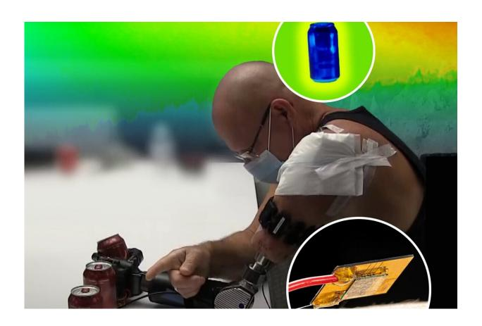
Johnny Matheny, a prosthetics tester, determines which cola can is the coldest using a modular prosthetic limb and thin-film thermoelectric device, both developed by the Johns Hopkins Applied Physics Laboratory. Credit: Ed Whitman / Johns Hopkins University Applied Physics Laboratory
