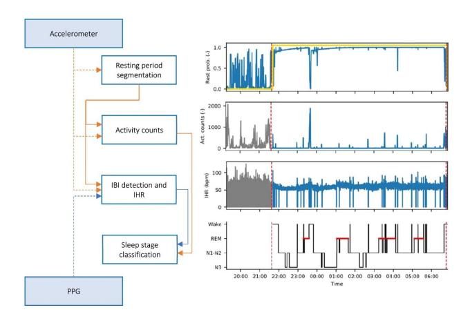
Overview of the processing steps for sleep stage classification based on accelerometer and PPG inputs; from top to bottom the plots represent: probability of the participant being at rest (in blue), and resting period found in the complete recording (in yellow), activity counts (in gray for the excluded period outside the resting period, in blue, during the resting period), instantaneous heart rate (idem), and predicted sleep stages; the vertical dashed
