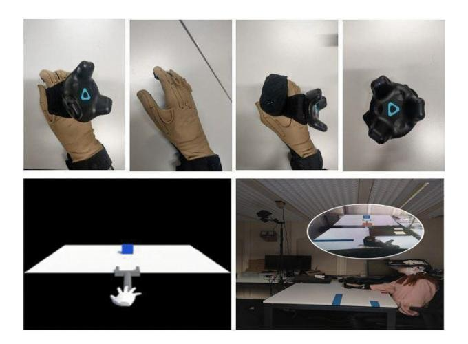
Experimental setup for tool-use training. Top row: CyberTouch-II and Wireless HTC Vive Tracker. Bottom row: Scene view. Credit: *Experimental Brain Research* (2023). DOI: 10.1007/s00221-023-06644-3
