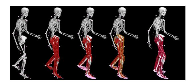
Schematic of the four steps involved in the model personalization process, from personalizing joint models, to muscle-tendon models, to ground contact models, to neural control models, resulting in a final personalized model that can be used to predict the patient's post-treatment walking function. Credit: Fregly group/Rice University
