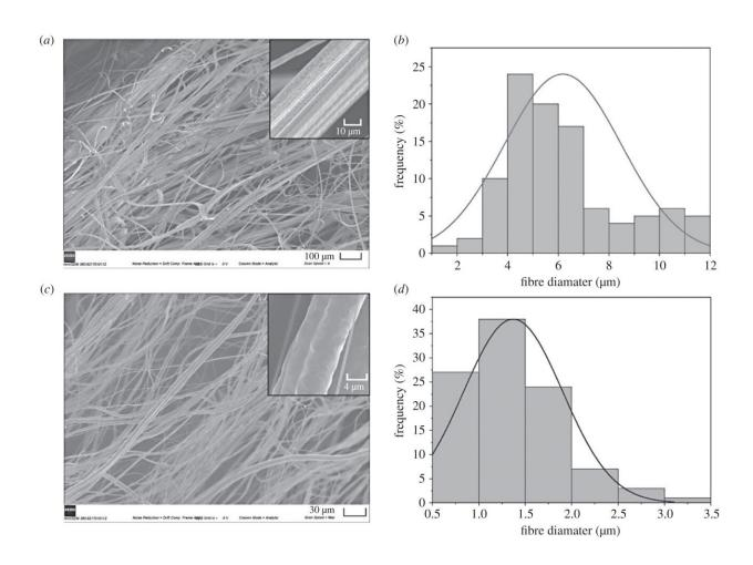
Scanning electron micrographs of: (a) virgin PCL fibers produced by pressurized gyration, including an inset to show fiber surface, and (c) casein-loaded PCL fibers including an inset to show fiber surface. (b,d) Respective graphs showing fiber diameter distribution, where n = 100 fibers. Credit: *Journal of The Royal Society Interface* (2023). DOI: 10.1098/rsif.2023.0166
