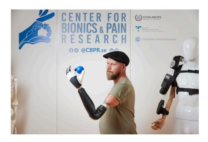
Patient wearing a prosthetic arm directly attached to the skeleton and neuromuscular system, which after surgical reconstruction of his residual limb, allows him to control individual fingers of a bionic hand. Credit: Chalmers University of Technology/Anna-Lena Lundqvist
