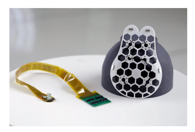
On the left of the photo, a yellow strip-cable has a green circuit board on one end, and a small ultrasound tracker on the other. On the right, the white device is teardrop shaped and has a hexagonal grid of holes where the tracker can be placed. Credit: Canan Dagdeviren
