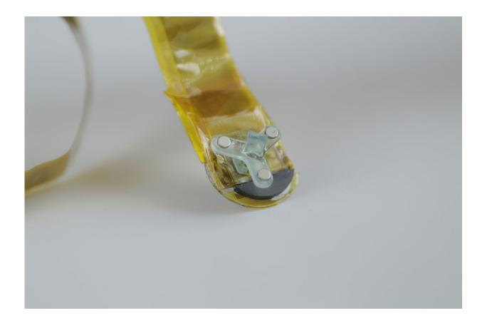
A close-up of the tracker shows that it is Y-shaped and has 3 metallic discs. The tracker is at the end of a yellow strip-cable. Credit: Canan Dagdeviren
