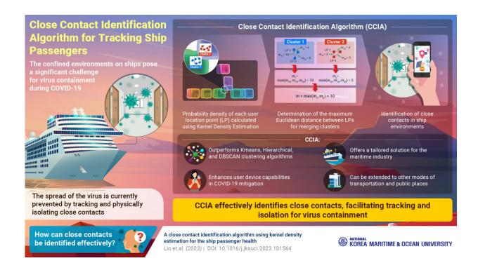
Researchers from KMOU have developed a novel algorithm that determines the Euclidean distance between user location points to effectively identify close contacts in confined environments (such as in ships), facilitating the tracking and isolation of potential virus spreaders. Credit: Professor Jooyoung Son from Korea Maritime and Ocean University
