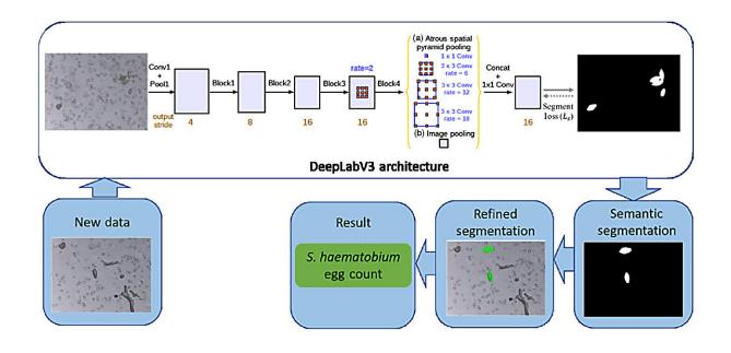
Schematics of the proposed two-stage diagnosis framework urogenital schistosomiasis with DeepLabV3-MobileNetV3 deep learning architecture for semantic segmentation of eggs and refined segmentation for overlapping eggs separation and count. Credit: *Journal of Medical Imaging* (2023). DOI: 10.1117/1.JMI.10.4.044005
