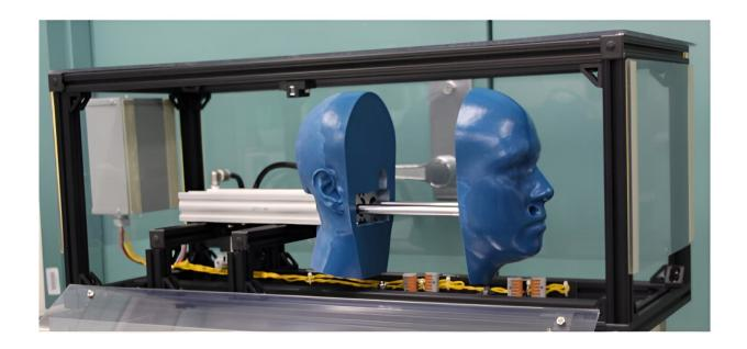
The team's mechanical test fixture that supports reuse testing, including donning cycles, speed, and mask displacement. Credit: Adam Hammond-Clements
