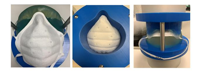
One of the first versions created by the team to test performance of a mask on a human face. The testing device drops down and compresses the mask with 50psi. Credit: Michael Omana
