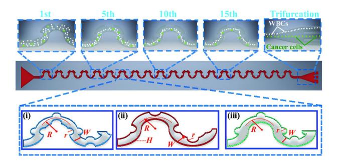
Schematics of particle unilateral focusing and separation in sinusoidal microchannels with asymmetric obstacles: (i) concave and convex obstacles on each respective sidewall (concave–convex obstacle channel), (ii) concave obstacles on one sidewall (one-sided concave obstacle channel), and (iii) convex obstacles on one sidewall (one-sided convex obstacle channel). Credit: *Cyborg and Bionic Systems* (2023). DOI: 10.34133/cbsystems.0036
