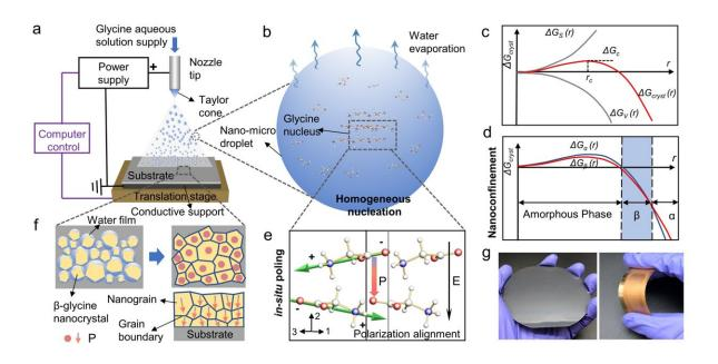
Fabrication of piezoelectric  $\beta$ -glycine nanocrystalline films and the active self-assembly mechanism via synergistic nanoconfinement and in-situ poling. Credit: HKUST
