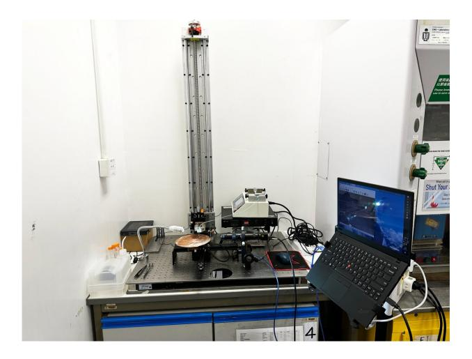
The bio-organic film printer (pictured) used to fabricate  $\beta$ -glycine nanocrystalline films was built by the research team. The printer and its relevant technique are US patent pending. Credit: HKUST
