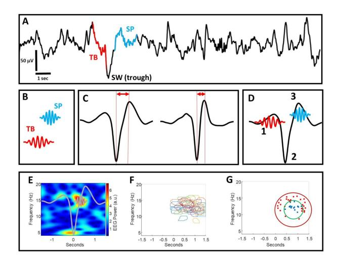
A) An illustrative example of raw sleep EEG data containing an identified theta burst (TB) event and a spindle (SP) event, each temporally coupled to the trough of a slow wave (SW) event. Note that not all SW events can be matched to
