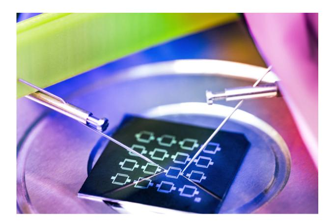
KAUST researchers have developed a sensor that can measure glucose levels in saliva, offering diabetics an alternative means to monitor glucose levels in their blood. Credit: 2023 KAUST; Anastasia Serin.
