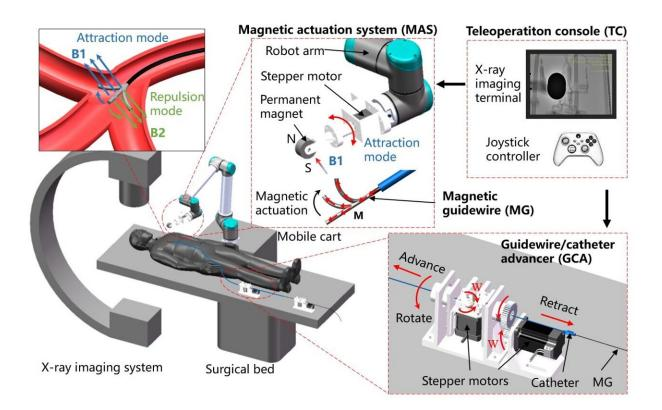
Schematic diagram of interventional surgery and the proposed magnetically controlled guidewire robot system (MCGRS). Credit: SIAT
