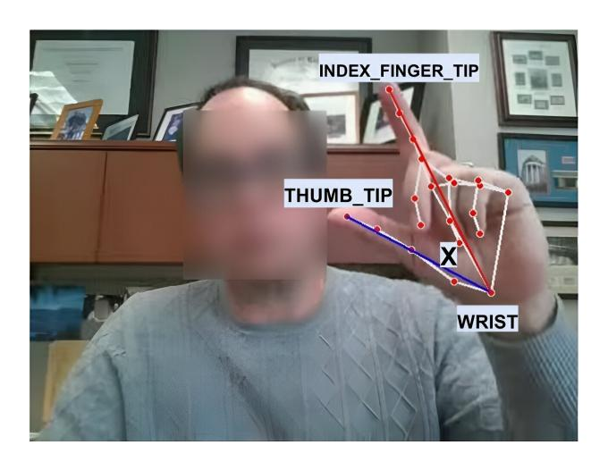
All the extracted key-points are displayed as red dots. The three key-points WRIST, THUMB\_TIP, and INDEX\_FINGER\_TIP were used to compute the finger-tapping angle X. Credit: University of Rochester / Saiful et. al.
