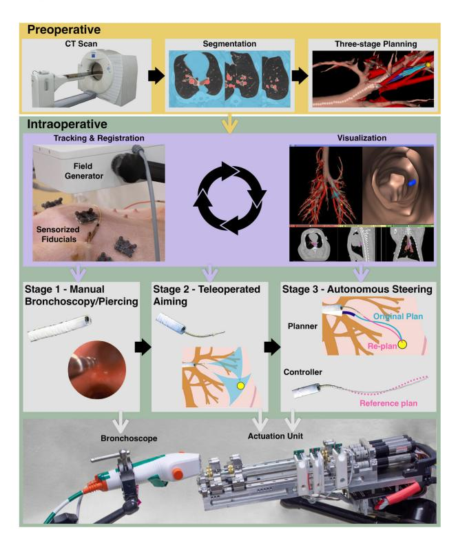
Workflow of the procedure showing the integration of the software and hardware components. We show both the procedure sequence flow (thick black arrows) and information flow (thin colored arrows). A CT scan was segmented and used to construct a map leveraged by the three-stage motion planning
