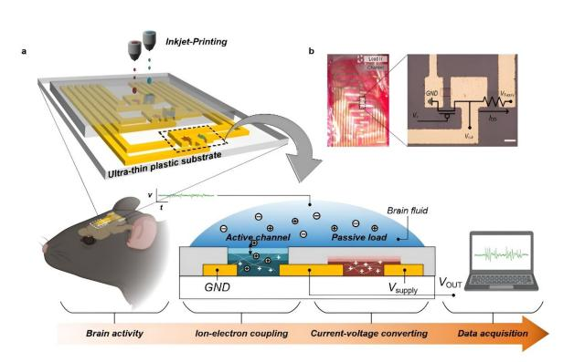
(a) Structure and functional mechanism of an implantable brain signal amplification sensor created using inkjet printing technology. (b) Magnified light micrograph displaying the sensor attached to the cerebral cortex (Left scale bar: 1, right scale bar: 100). Credit: POSTECH
