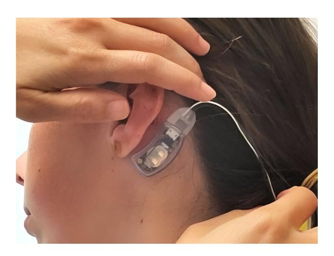
The IB-Stim device is placed near the ear and sends electrical impulses to nerve bundles. The nerves then activate brain areas involved in processing pain, rerouting the "pain pathways." Credit: University of California, San Francisco
