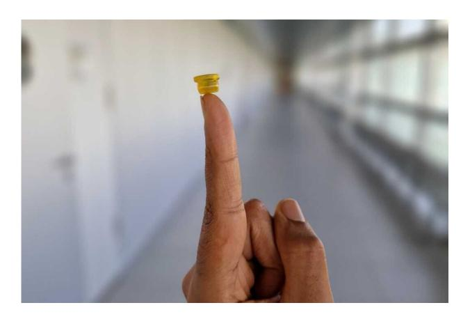
The suction cup measures around ten millimeters in diameter and six millimeters in height. Credit: Transire Bio
