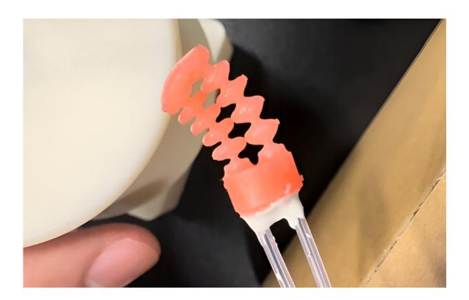
Air pressure within the two channels of the robotic catheter tip determines whether it deflects left or right. Credit: Noah Barnes, PhD Student, Department of Mechanical Engineering, Johns Hopkins University
