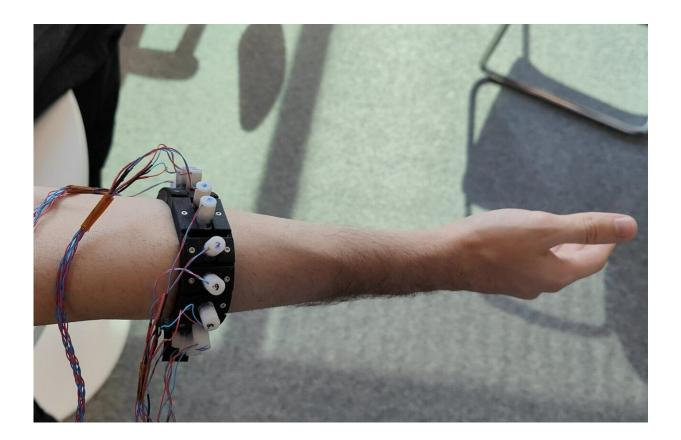
Sensor wristband demonstrator used to measure muscle activity relating to hand movements on test subjects. Credit: Fraunhofer IBMT
