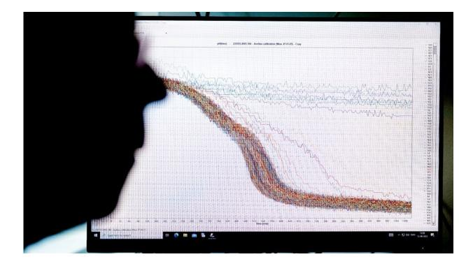
The scanner registers the color of each of the small wells and then graphs are calculated that show the extent to which each drug sours the milk. Credit: Bax Lindhardt
