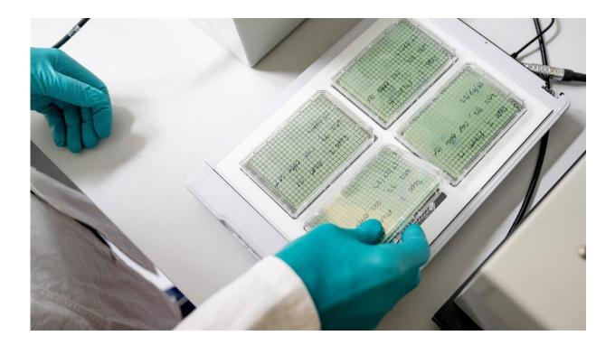
The plates with pharmaceuticals in each of the small wells are placed on the scanner. Egon Bech Hansen has added skimmed milk inoculated with a bacteria—the milk is colored blue by a pH indicator. When the milk sours, it changes color to greenish and the wells where the color is still blue indicates that the substance inhibits the acidification. Credit: Bax Lindhardt
