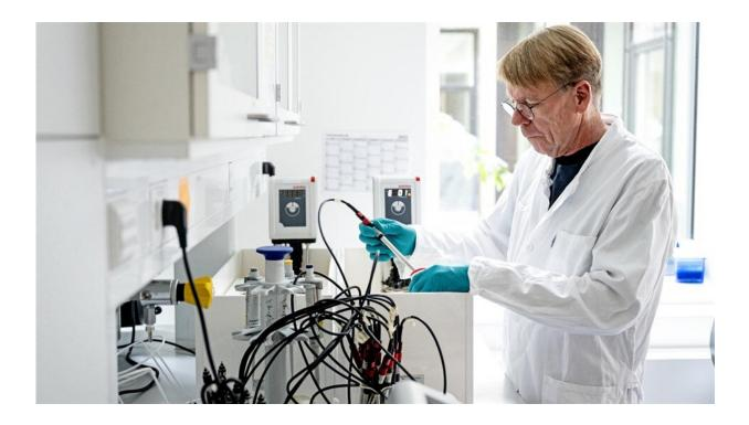
Before using the scanner, Egon Bech Hansen used a so-called pH electrode to register whether the milk soured. The setup with 16 electrodes takes up more space than the scanner with 4 x 386 wells. It would take 100 days to complete a similar experiment with pH electrodes—and would require much larger amounts of material. Credit: Bax Lindhardt
