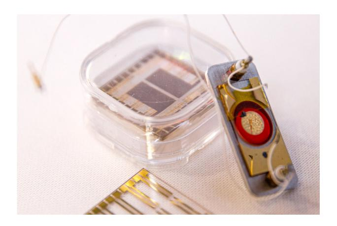
The Electronic Polymer Dosimeter for Radiotherapy, created by a team at Sandia National Laboratories. Credit: Spencer Toy
