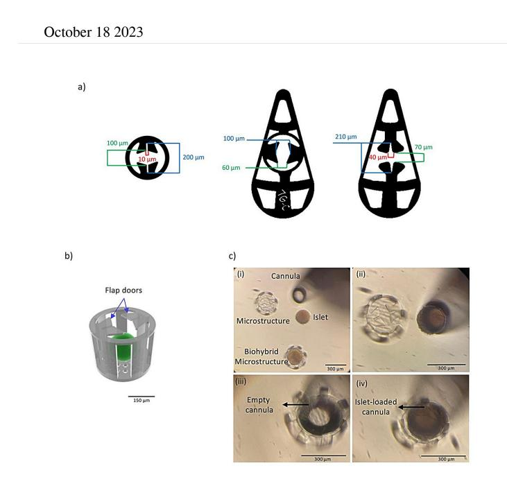
Microstructure design and islet localization procedure. (a) Schematic illustration showing the different designs of flap door feature applied in this study. (b) The
